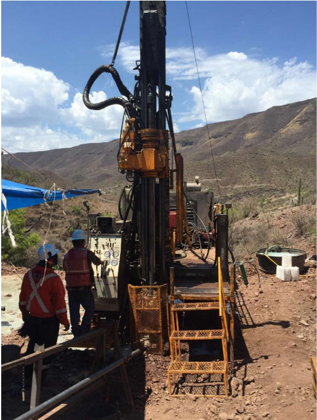
Figure 10.1.1: 2016 Toro Drilling Rig Producing NQ Drill Core
