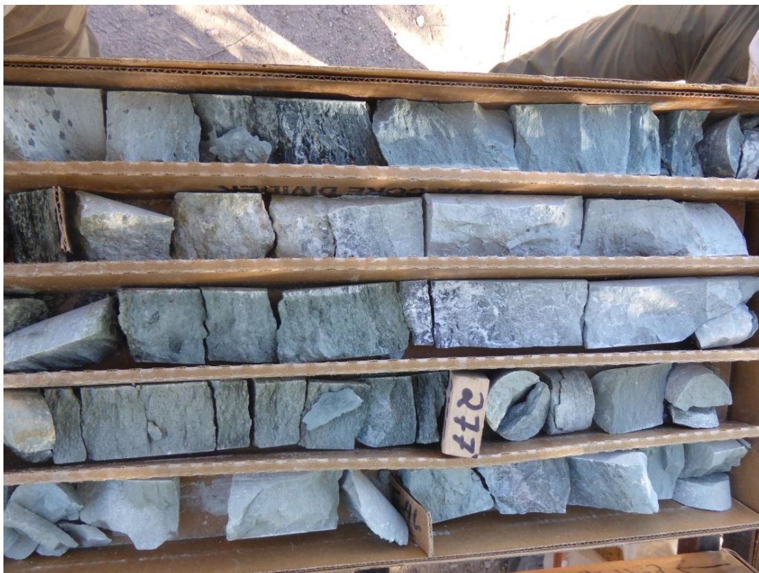
Figure 10-2: Drill core presented after cut and sampling procedures
