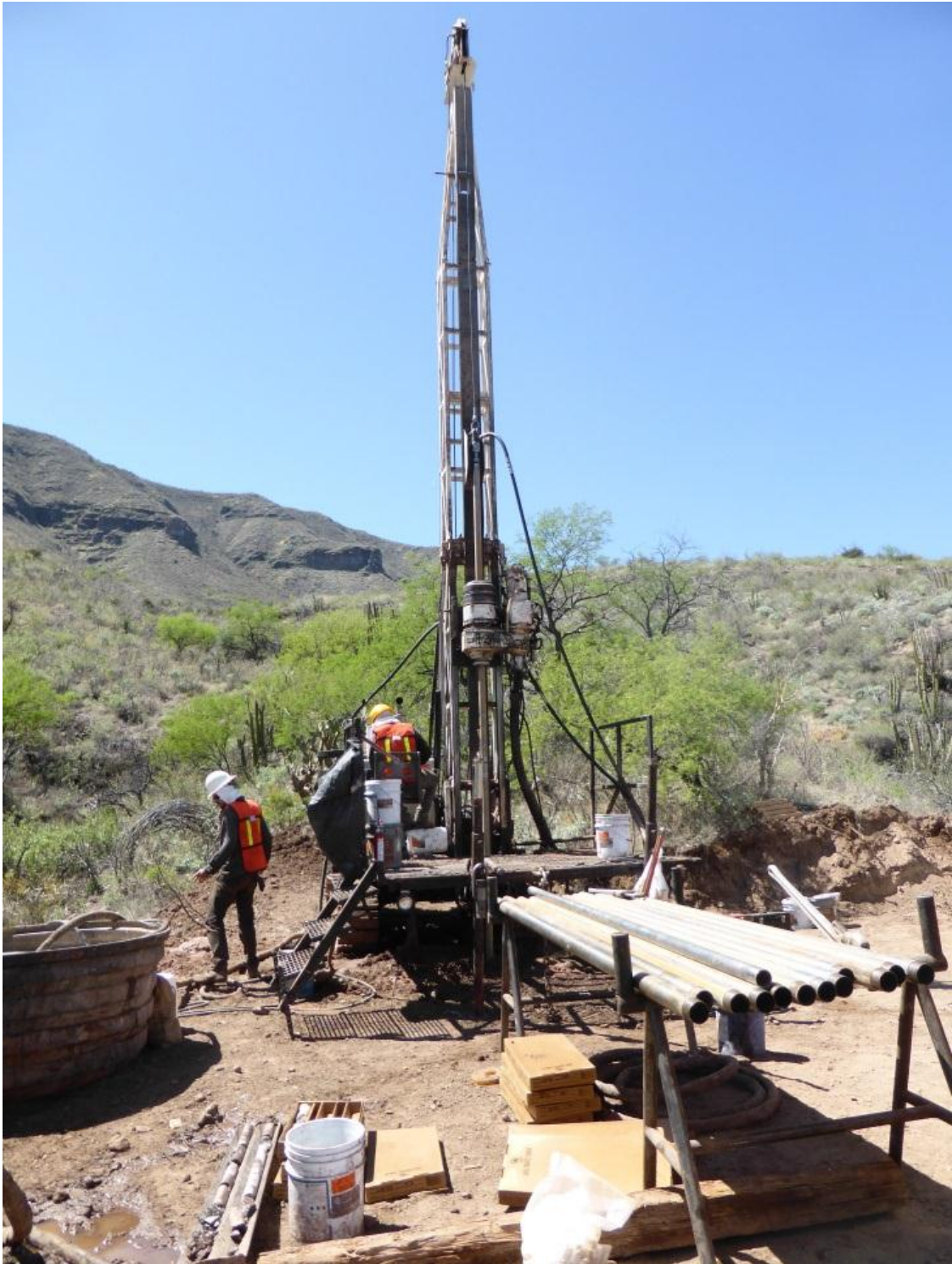
Figure 9-1: 2015 drill rig producing NQ drill core
