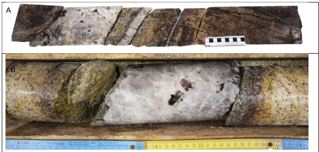
Figure 22: Representative drill core images of intersected vein mineralization (A) One major and several sub-veins of quartz and wolframite in the wall rock of the Teplice rhyolite (TR) (ZGLi 01/2012 – 71.0 to 71.75 m), (B) Typical “Flöz” vein hosted in Zinnwald albite granite (ZAG) showing narrow seams of adjoining greisenization (ZGLi 01/2012 – 88.0 to 88.45 m)
