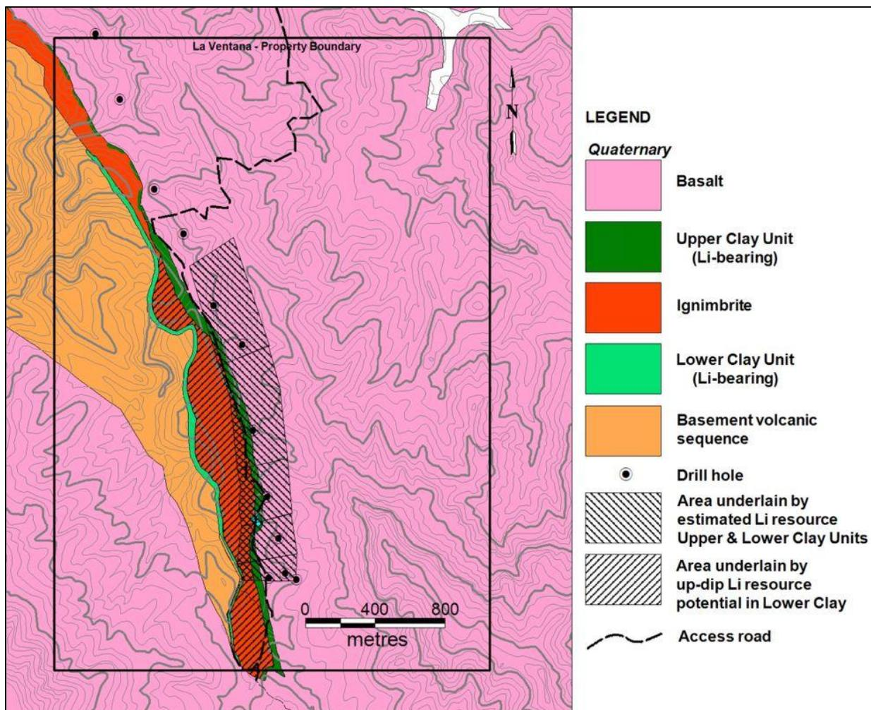
**Figure 13. Plan of Polygons used in La Ventana Inferred Resource Estimate**
