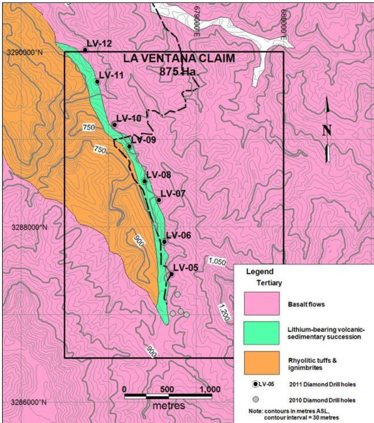
Figure 10. Location Plan of 2011 Drill Holes – La Ventana Concession.
