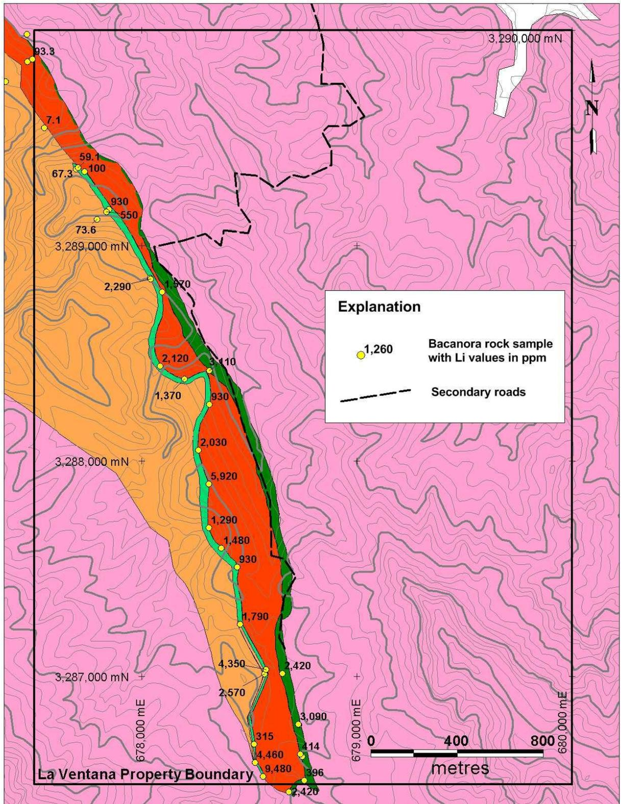
**Figure 8. 2012 Rock Sample Location Plan - La Ventana Concession.**
