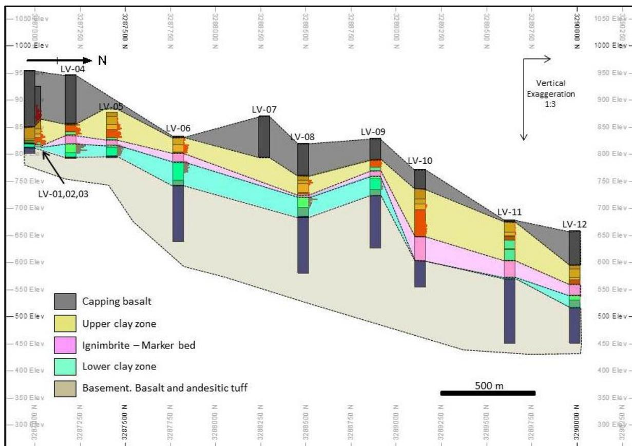
Figure 11. Geological Long Section through the 2011 Drill Holes.
