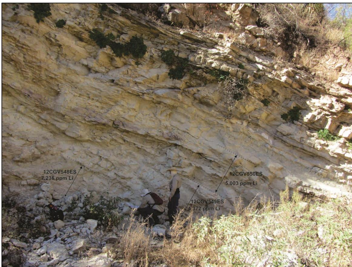
**Figure 14. El Sauz concession Li-bearing clay unit**
