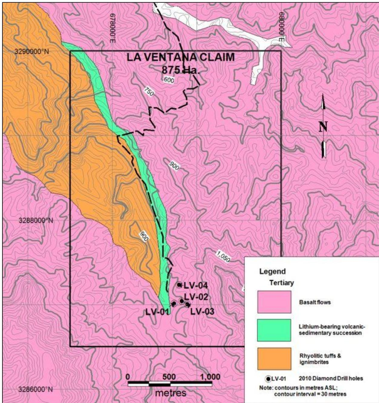
**Figure 9. Location Plan of 2010 Drill Holes – La Ventana Concession.**
