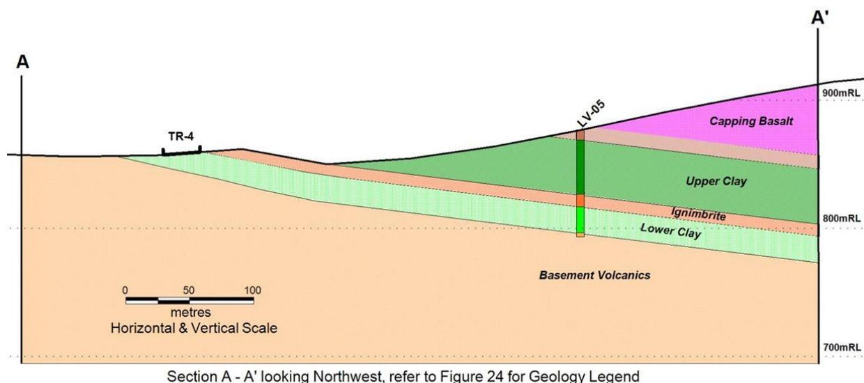
**Figure 12. Cross Section through Drill Hole LV-05 and Trench TR-4**
