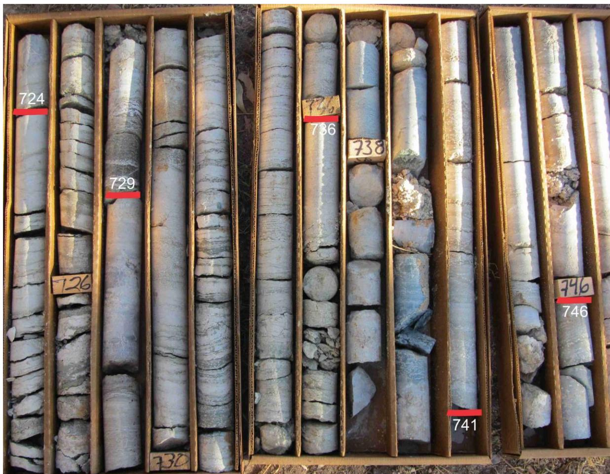
Figure 18. Hole ES-02 Lower Clay unit intercept from 722 to 752 feet.
