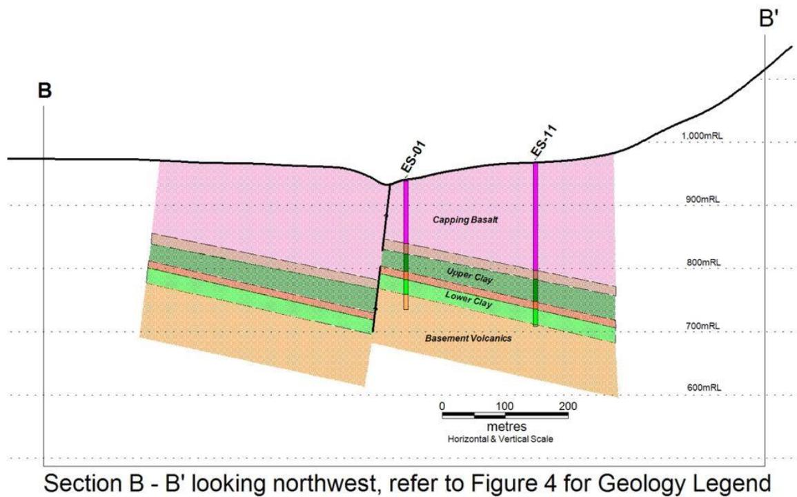
**Figure 15. Cross Section through Drill Holes ES-01 & ES-11.**
