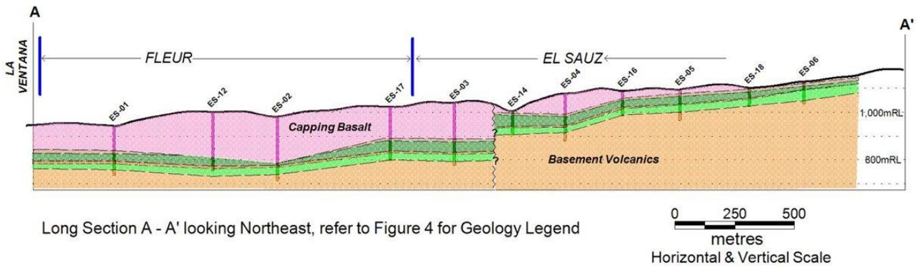
**Figure 14. Long Section through drill holes ES-01 to ES-06.**
