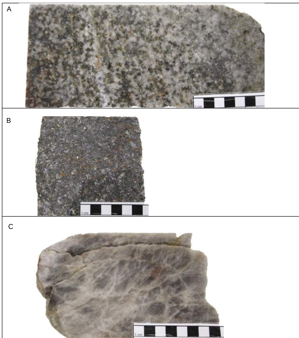
Figure 18: Representative drill core images of the prevailing three greisen types occurring in the Zinnwald deposit (A) Predominant quartz-mica greisen (ZGLi 01/2012 – 108.0 to 108.25 m), (B) Quartz-poor mica greisen rich in purple fluorite (ZGLi 02-2012 - 97.9 to 98.0 m), (C) Quartz greisen (ZGLi 02/2012 – 189.85 to 191.0 m)
